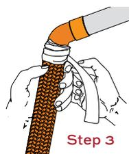
4. Direct the torch away from the base of the copper fitting and braided section. Avoid contact of the flame with the base of the copper fitting and braid. Heat end of copper fitting for proper flow of silver solder. Silver solder flows at approximately 430°F (221°C).
