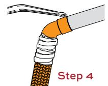
5. Use caution with brazing rod or other higher temperature techniques. Overheating will cause leaks.
