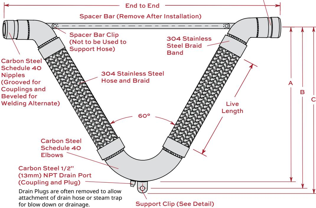
Our steam service ratings are very low in the interest of safety although our 70°F (21°C) pressure ratings are as high or higher than our competitors. All locations where failure could lead to personal injury or suffocation must be avoided. In dangerous locations we suggest housed expansion joints, solid loops, ball joints, packed devices etc. rather than thin walled flexible products regardless of manufacturer.
