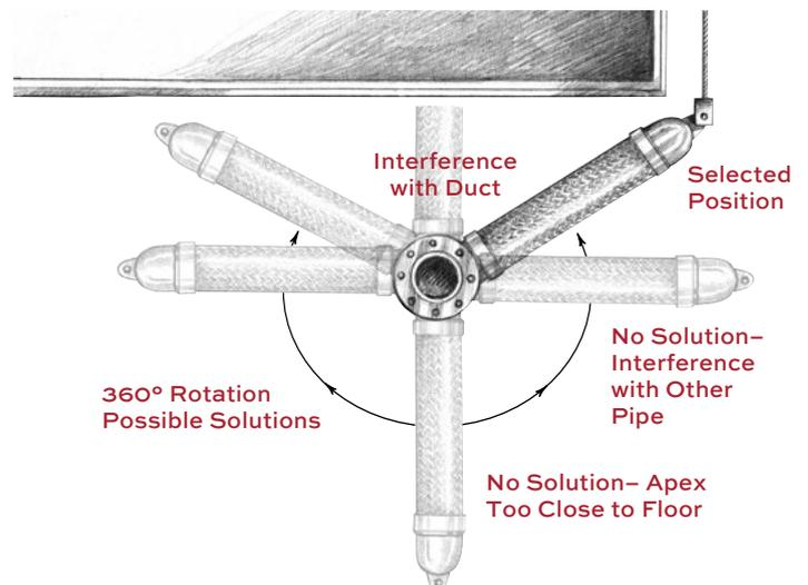
Our standard vee allows for 4" of seismic motion in all directions. The design is very conservative and in expansion locations with no change to the standard product we agree to 6" movements, when the movement is axial compression and extension.
