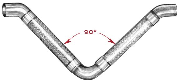
In fairness to others, we should note that all these hose designs can be made to work, if the hoses are made long enough to keep stress within acceptable limits for the stated movements.
