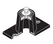
Type ND neoprene mounts are designed for simple installations. The rubber is loaded in both shear and compression to provide the desirable straight line rubber-in-shear deflection curves as well as overload protection. They are molded assemblies with skid resistant rubber ribbed baseplates and need not be bolted to the floor on most installations. Maximum deflection is 0.5".
